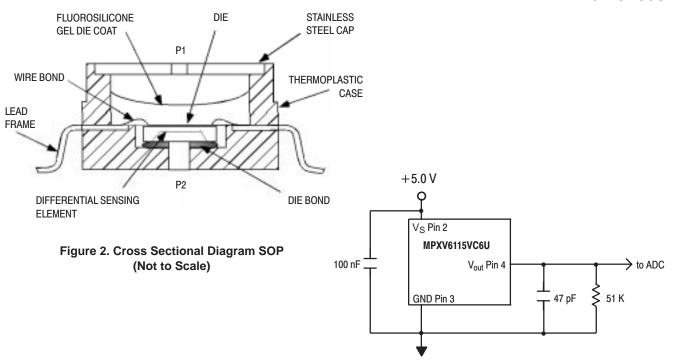
Figure 3. Typical Application Circuit (Output Source Current Operation)
