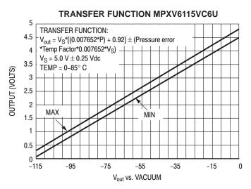
Figure 4. Output versus Absolute Pressure
