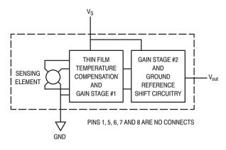
Figure 1. Fully Integrated Pressure Sensor Schematic
