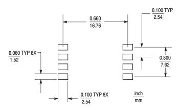
Figure 5. SOP Footprint (Case 482A)
